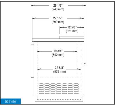
$\underline{\textbf{IMPORTANT NOTE}}\text{: A $\underline{\text{minimum clearance of 3"}}$ is $\underline{\text{required}}$ on each side, front and rear of cabinet for optimum performance.}$
